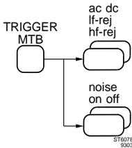
Toggle softkey to select MTB trigger coupling modes ac, dc, lf-reject, and hf-reject.
