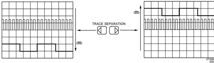
**NOTE:** There is a second way to operate the trace separation. If the DELAYED TIMEBASE menu is activated you will see the 'T' symbol next to the TRACE SEP text. The 'T' indicates that the cursor TRACK control can be used to adjust the trace separation.
