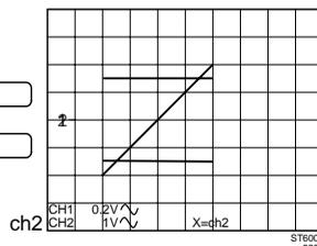
The diagonal line (ch2 against ch2) is the result of XY display of two equal signals without phase shift. Phase shift will result in an elips or even (90° phase) in a circle.
