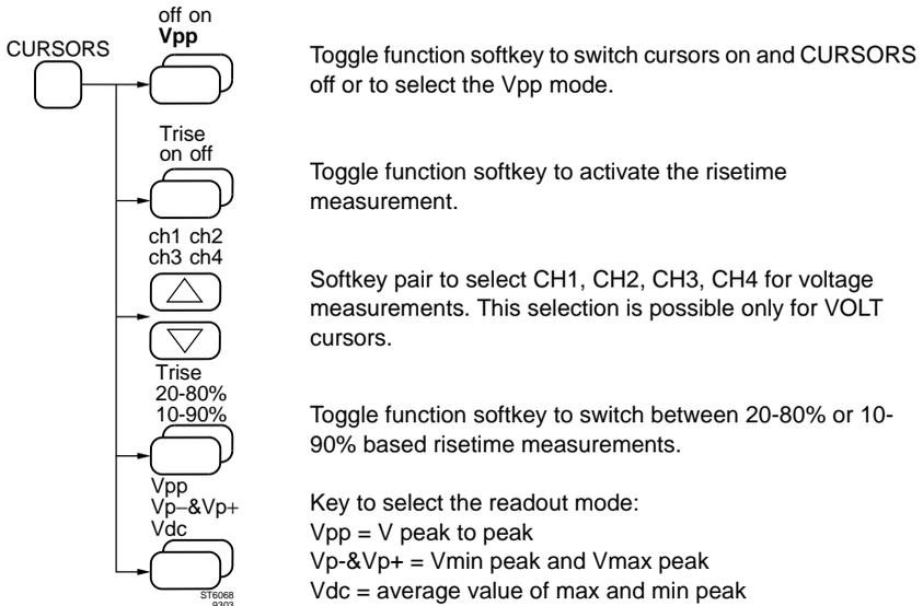
The average value of the measured maximum and minimum peak is displayed in the Vdc mode. This readout mode can be used to measure dc components of symmetrical signals and true dc signals.
