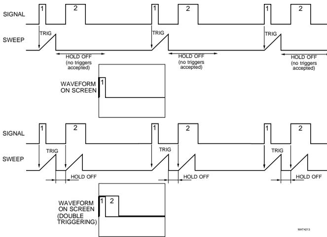
Using HOLD OFF to suppress double triggering
