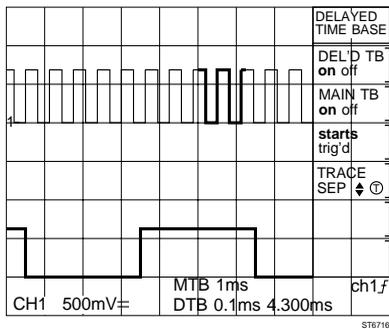
The main timebase trace and delayed timebase trace are displayed simultaneously.
