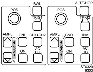
The CH1 and CH2 section of the PM3084 is shown on the left.
