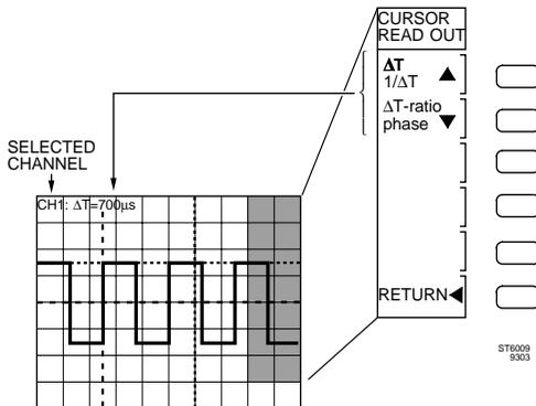
$\Delta T$  is the time difference between the time cursors. The readout is in seconds (s), or fractions thereof.
