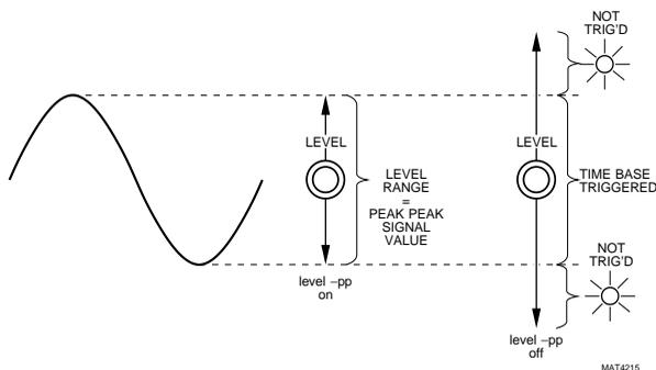
MTB LEVEL control ranges in level-pp on and off
