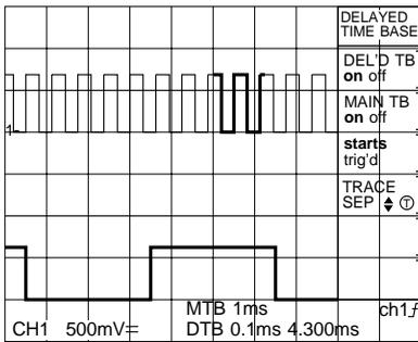
In the menu you will find a 'starts/trig'd' softkey. Starts is highlighted indicating that the delayed timebase is operating in the starts mode instead of the triggered mode.
