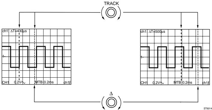
At the top of the screen, the time distance between ( $\Delta T$ ) is displayed. This is used for timing measurements.
