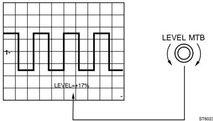
Observe that the primary trigger functions (source, slope and level) have direct access keys. For most day to day applications, menus are not needed.
