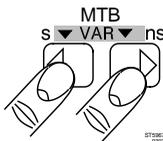
Fine adjustment of time base speeds between the 1-2-5 steps of the can be made by pressing the MTB key pair for MTB VAR. In the VARIable MTB mode the timebase readout gets a higher resolution.
