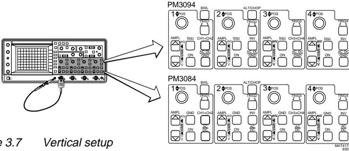
Figure 3.7 Vertical setup
