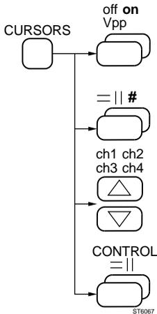
Toggle function softkey to switch between cursors on, off or Vpp mode.
