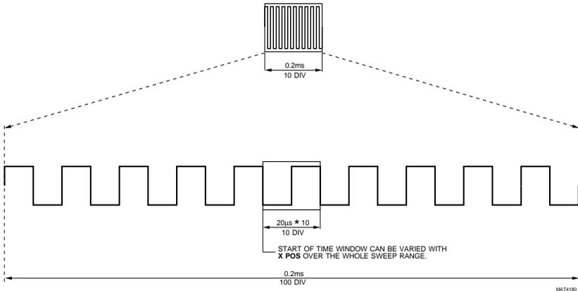
Function of timebase magnifier and X POS control
