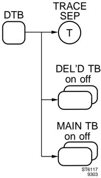
The 'T' symbol in the menu indicates that the TRACK cursor control can also be used for adjusting the TRACE SEparation when the menu is displayed.
